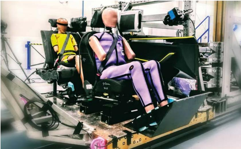
assessments of automotive safety systems and components. In the area of safety related to side impact collisions, active lateral intrusion simulation (ALIS) testing systems are available to assess the performance of critical vehicle safety components in physical simulations of side impact crashes. These advanced, non-destructive DYCOT systems can be particularly useful in evaluating the performance of passenger restraint systems including frontal and side airbags.
