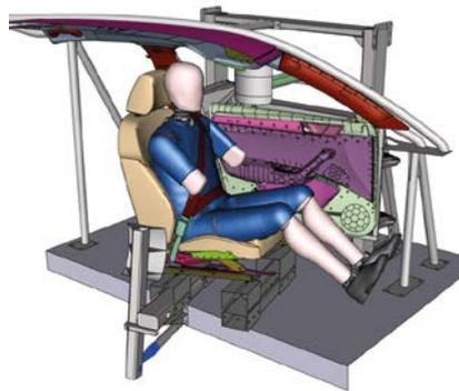
Multiple displacement actuators can be applied in a wide range of configurations along the side of the facsimile vehicle under test, allowing technicians to simultaneously evaluate the results of simulated side and pole impact for both front
