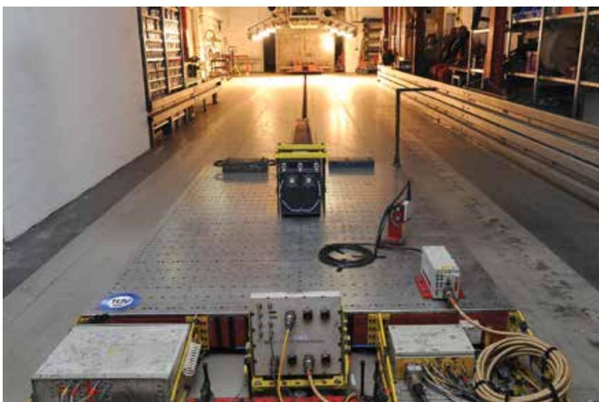
Battery module being prepared for a mechanical shock test.
