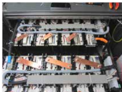
Figure 2: Reassembled second life battery pack
