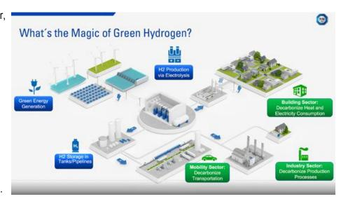
As a storage medium, it can be used to balance fluctuations in electricity production from renewable sources of energy. Hydrogen further establishes a link between electricity, heat and gas networks, the transport sector and industry.
