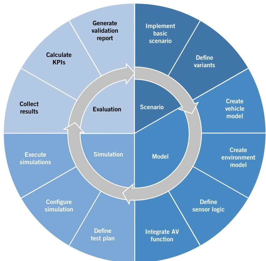
**FIGURE 1** Virtual validation process for automated driving functions (© TÜV SÜD)
