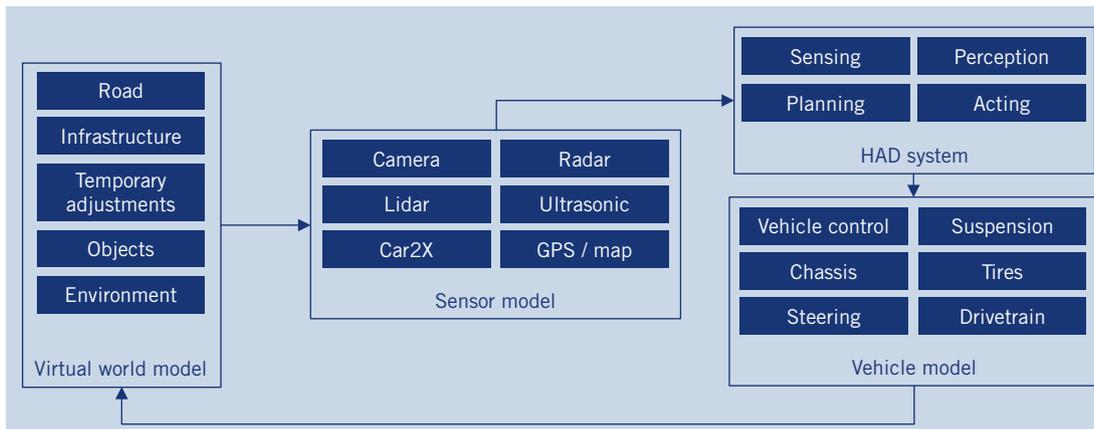
**FIGURE 3** Modular model structure guarantees universality of the method (© TÜV SÜD)
