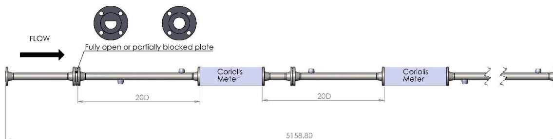
Figure 2. The 2-inch metering setup.
