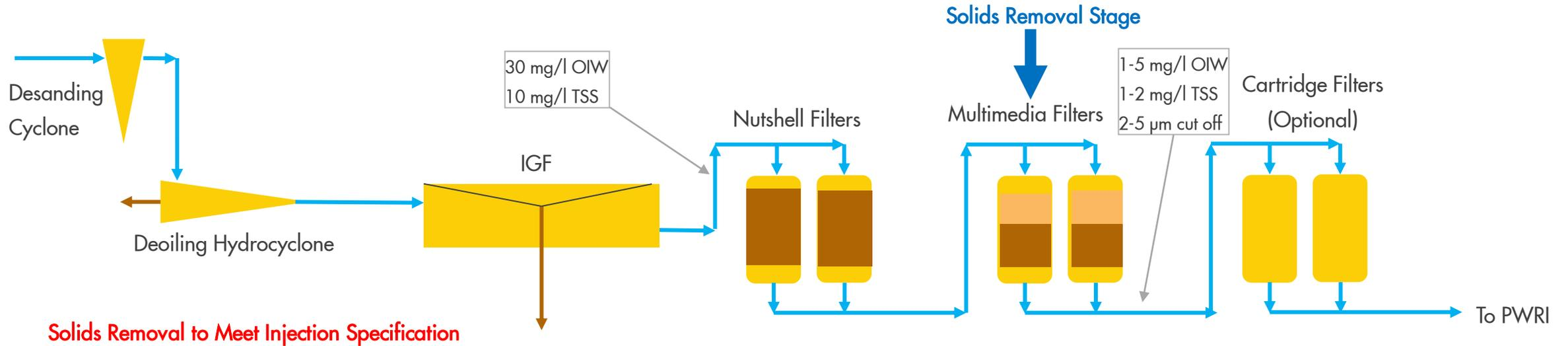
Solids Removal to Meet Injection Specification
