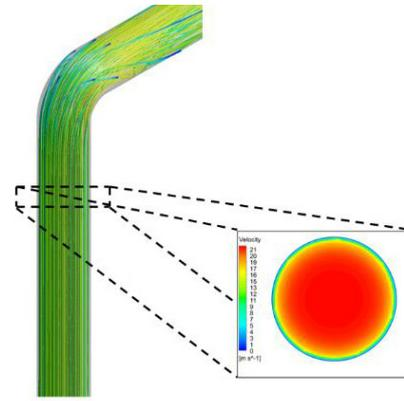
Figure 2: Example of Flow Profile Downstream of In Plane Bend (only a small deviation from fully developed flow)
