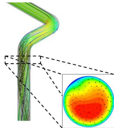
Figure 3: Example of Flow Profile Downstream of Out of Plane Bend
