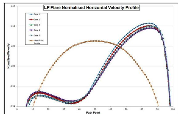
Figure 4: Example of Ideal Flow Profile vs As Found Profile At The Meter
