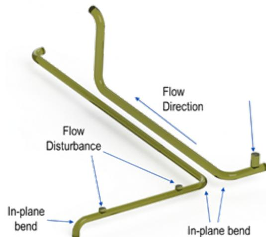
Figure 1: CAD Model of A Typical Flare Metering Line
