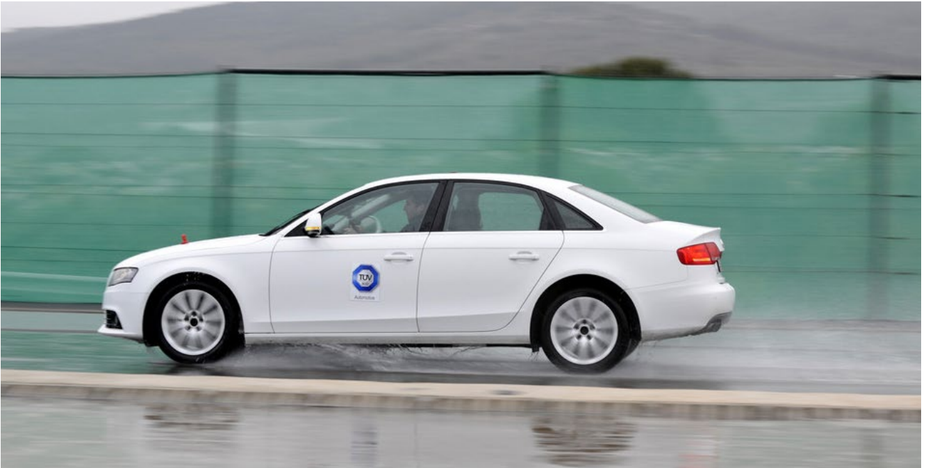
Figure 8: Wet grip measurement - vehicle method
