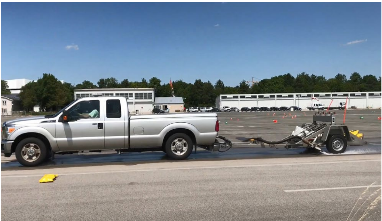
Figure 7: Wet-grip measurement - trailer method
